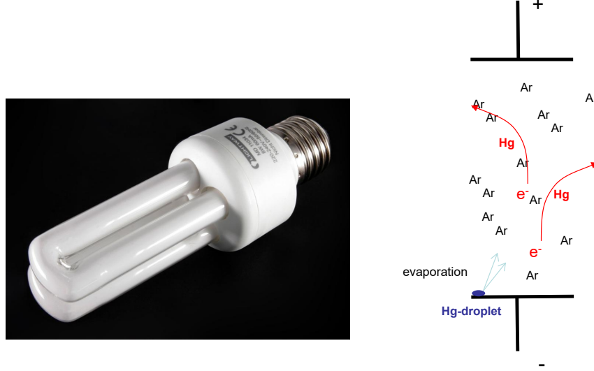
Figure 3.8: Adding mercury to an energy-saving lamp increases the electrical resistance of the plasma and thus the dissipated power in the plasma itself. With this dissipated power, the light output simultaneously increases.
